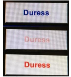
Three different images capturing the three potential states of the Duress alarm indicator in the Z Building Booth. During normal operations, the top icon is shown. When the duress alarm is triggered, the icon will change back and forth between the middle and bottom image. This is the only indicator on the main screen of the booth that an alarm has been triggered. This rectangle is approximately 1.5 inches long.
